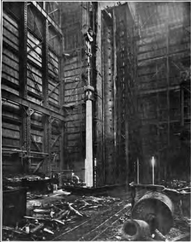
GUN TUBE READY FOR QUENCHING.
