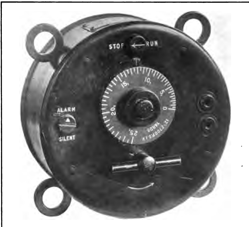
TIME OF FLIGHT CLOCK WHICH RINGS A BELL WHEN THE SALVO IS ABOUT TO FALL, THEREBY ASSISTING THE SPOTTER TO IDENTIFY THE SPLASHES FROM THE GUNS HE IS OBSERVING.
