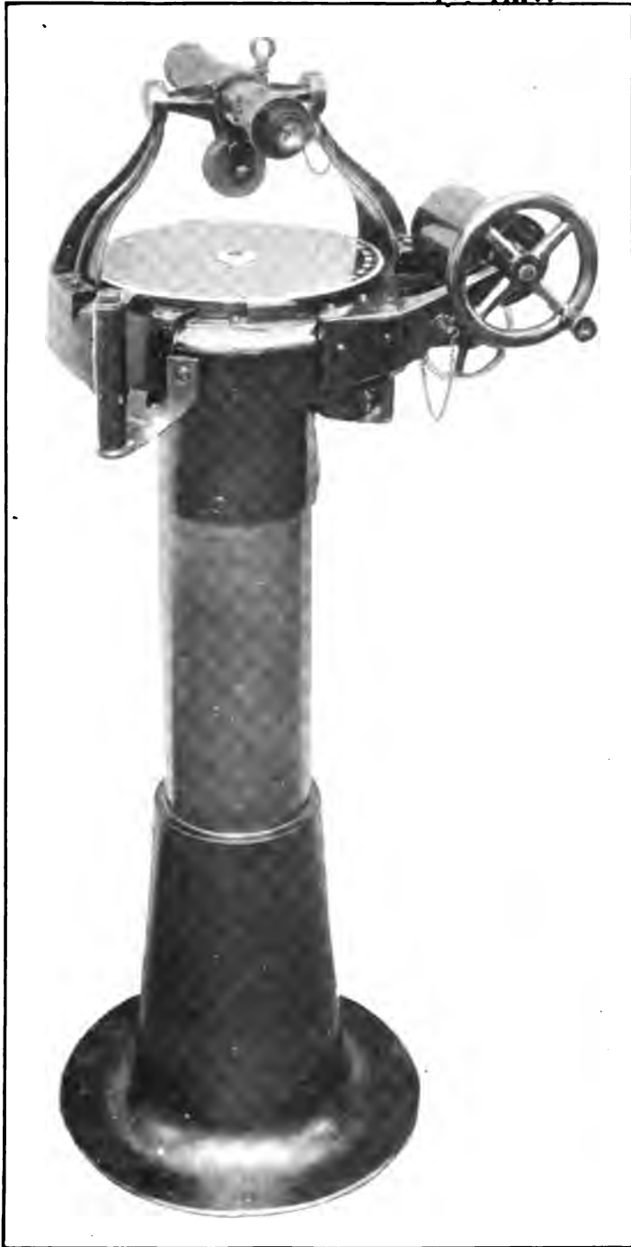
TARGET-BEARING TRANSMITTER WHICH TRANSMITS THE BEARING OF THE ENEMY TO PLOTTING ROOM AND GUNS.
