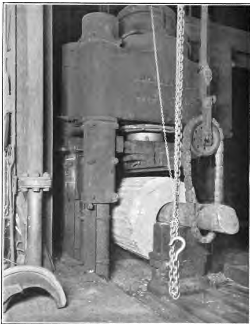
FORGING A GUN JACKET IN A 2,500-TON PRESS.
