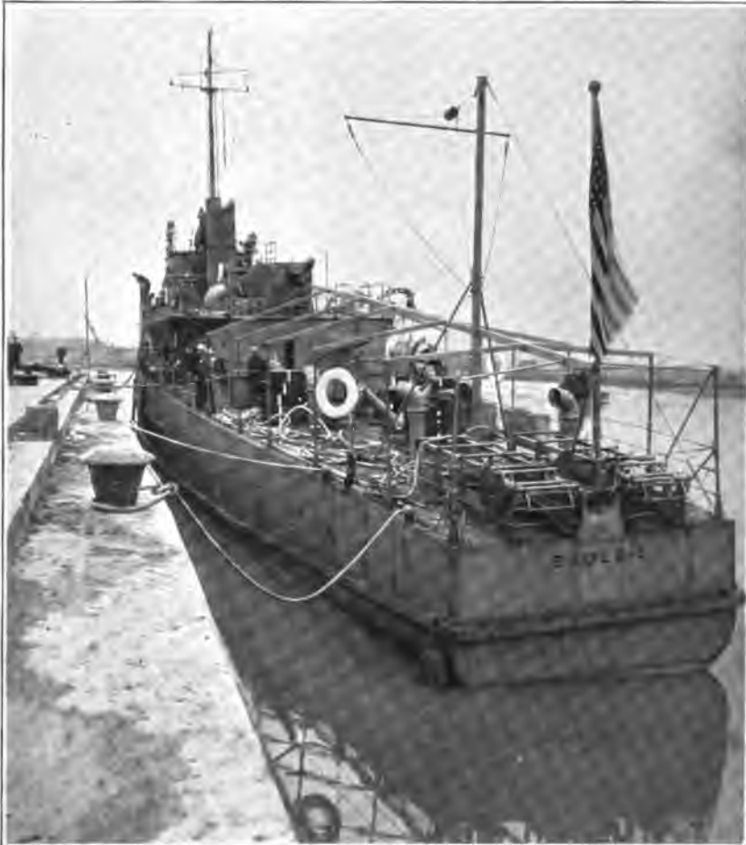
U. S. PATROL BOAT EAGLE 1, SHOWING DEPTH-CHARGE LAUNCHING GEAR AT STERN, "Y" GUN AMIDSHIPS, AND STERN GUN ON DECK HOUSE.
