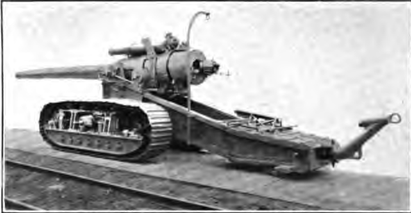
7-INCH GUN ON CATERPILLAR MOUNT (WEIGHT, 76,000 POUNDS) ON FIRING POSITION. BREECH OPENED, GUN READY TO LOAD.
