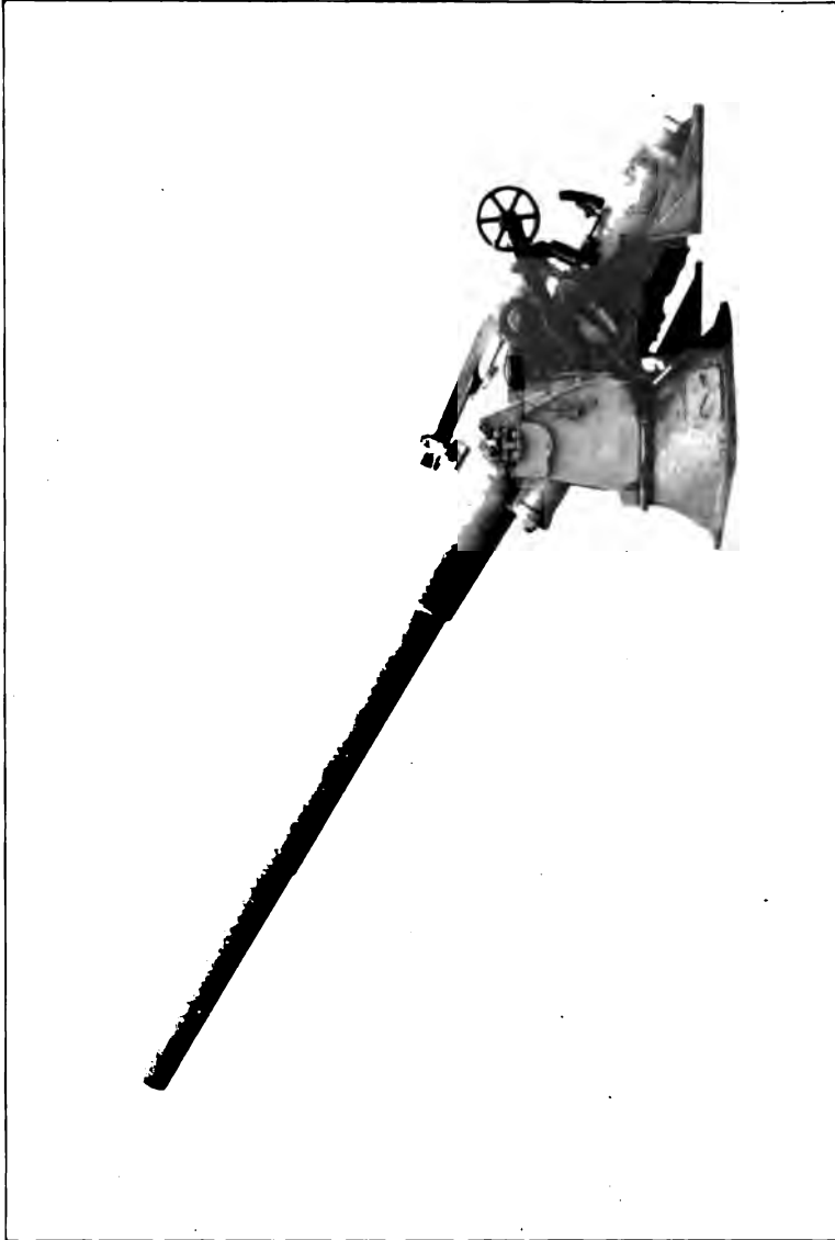
A 6-INCH 40-CALIBER GUN MOUNT AT 30° ELEVATION. This mount originally had a maximum of but 15° elevation and was the first mount modified at the New York Yard.
