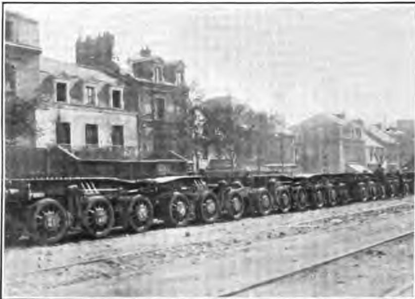
TRUCKS FOR 14-INCH RAILWAY BATTERY GUN CARS LINED UP ALONGSIDE OF DOCK AWAITING UNLOADING OF GIRDER.
