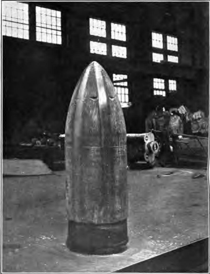
MIDVALE NAVAL 14-INCH ARMOR-PIERCING PROJECTILE AFTER PENETRATING A 13½-INCH CLASS A ARMOR PLATE.
