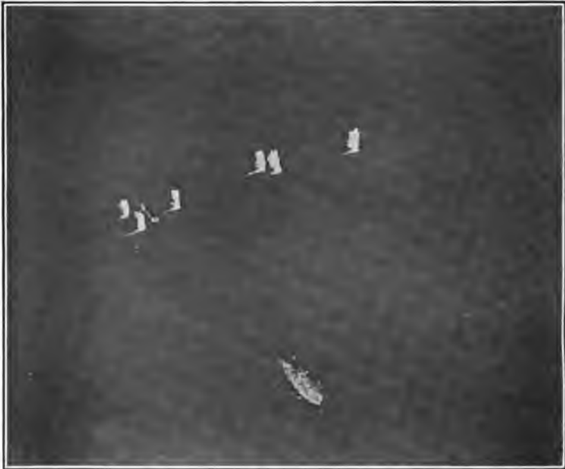
SALVO "STRADDLE," OBSERVED FROM A SEAPLANE. TOWING SHIP IS 400 YARDS FROM TARGET.
