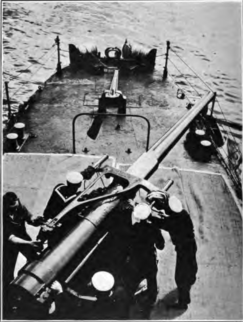
STERN OF A DESTROYER, SHOWING GUN CREW AT STATIONS AND TWO DEPTH CHARGES READY FOR LETTING GO.
