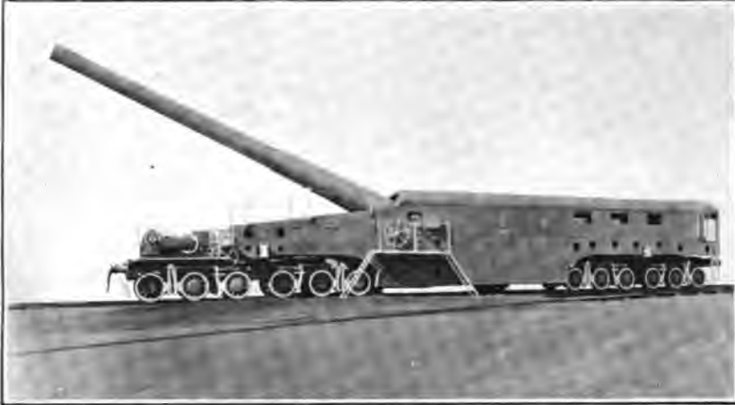
14-INCH GUN ON RAILROAD GUN CAR. TYPE USED ON WESTERN FRONT BY U. S. NAVY.
