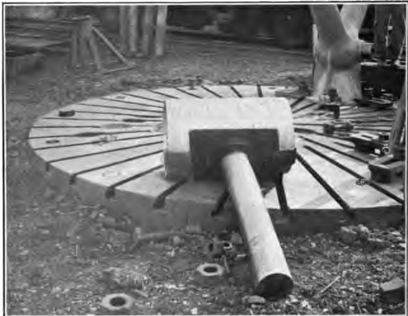
PROJECTILE FOR "Y" GUN, SHOWING DEPTH CHARGE ATTACHED TO ARBOR.
