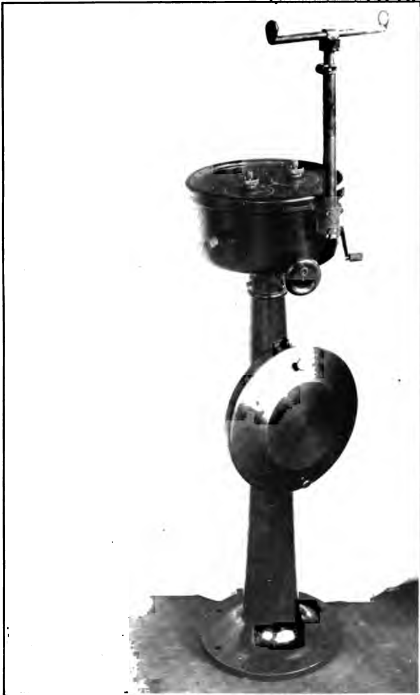
FORD RANGE KEEPER, MARK II, FOR USE WITH TORPEDO DEFENSE BATTERIES AND ON SMALL VESSELS.
