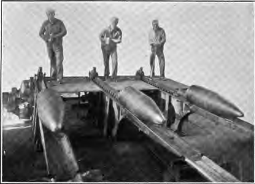
BATTERY OF RAMMERS FOR A 3-GUN TURRET READY FOR SHOP TEST.
