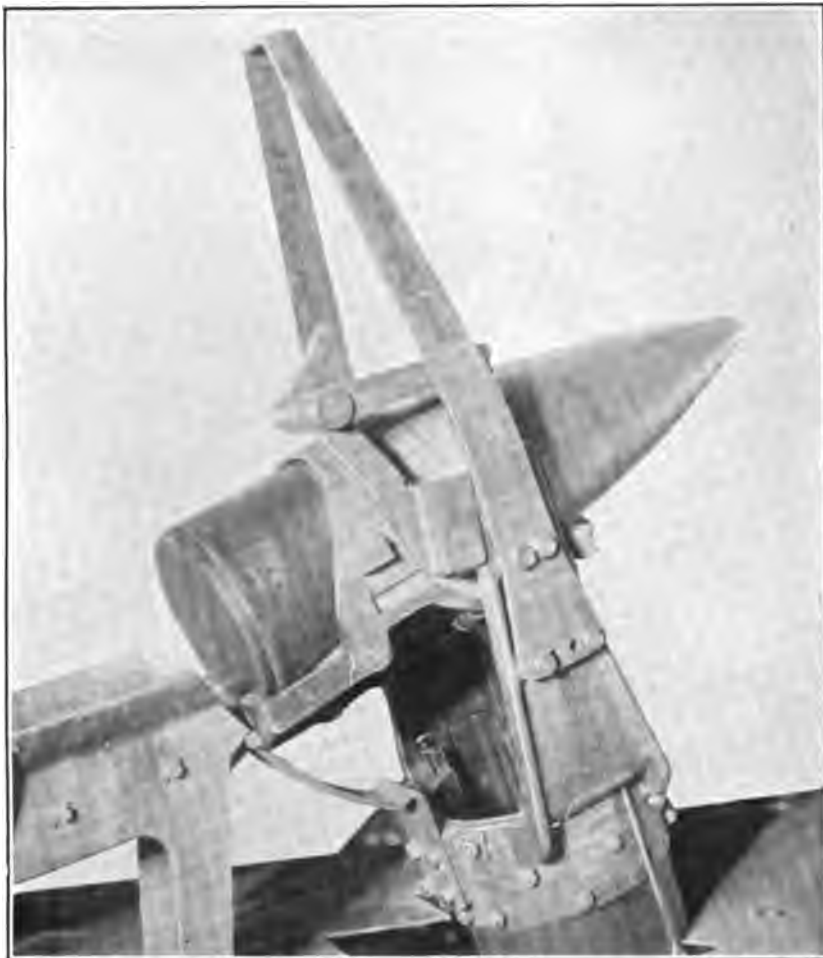
14-INCH PROJECTILE IN CRADLE BEING SMLIC TO LC/DING FLATCFM.
