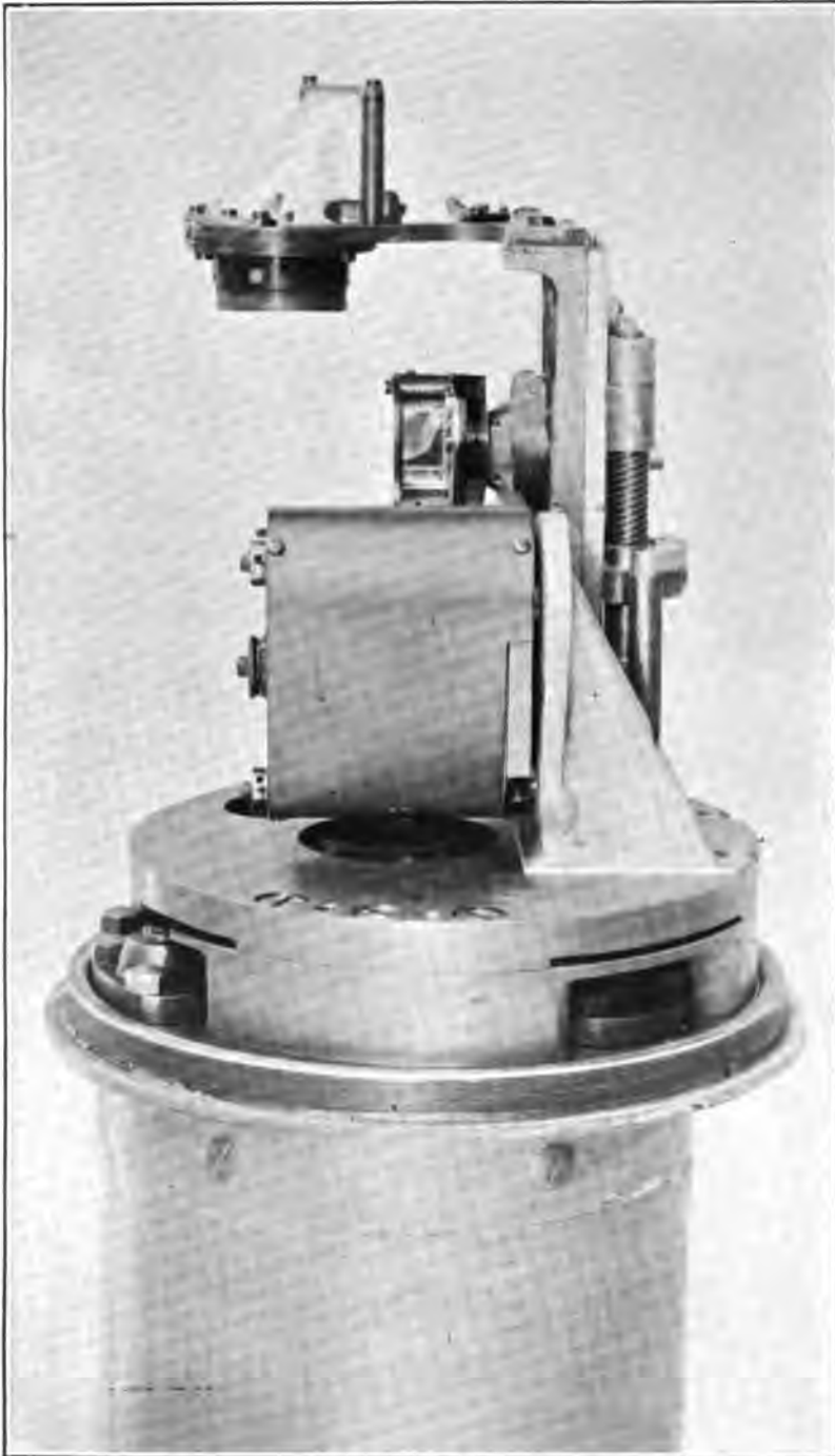
END BOX REMOVED FROM RANGE FINDER, SHOWING MOUNTING OF END PRISMS. All prisms, lenses, and mirrors must be in exact position, and all mechanical fitting must be within the smallest possible tolerance in order that the instrument function properly.
