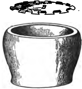
FIG. 167.—LAG DRAWN IN FOR BOTTOM.
