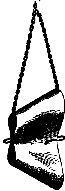
FIG. 402.—SHOWING PATTERN DOUBLED UP.
