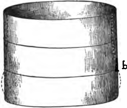
FIG. 166.—MANNER FOR RAISING TOP PART OF BODY.
