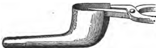
FIG. 87.—MANNER OF HOLDING SPOUT WITH TONGS.
