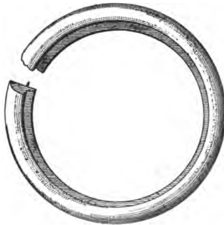
FIG. C.—RING FOR COVER SUPPORT.
