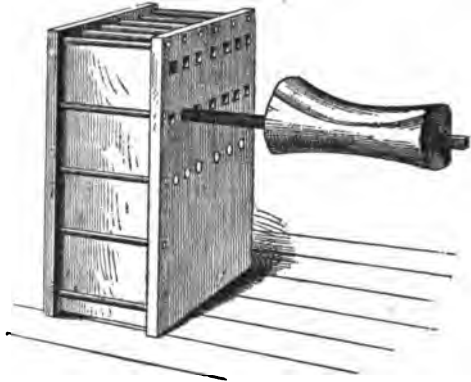
FIG. 411.—MANDREL FOR PLANISHING BELL.
