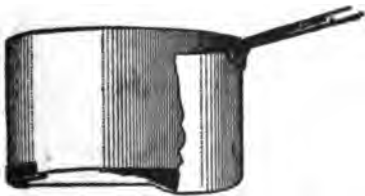
FIG. 10.—PIECE PUT THROUGH OUTSIDE.
