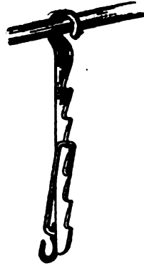
FIG. 191.—POT HOOK AND RACK.
