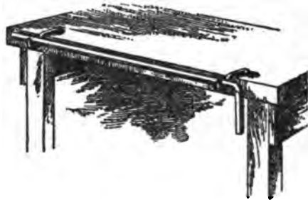
FIG. 25.—MANDREL IN POSITION.
