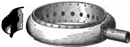
FIG. 299.—SECOND FORM OF FIRE POT.
