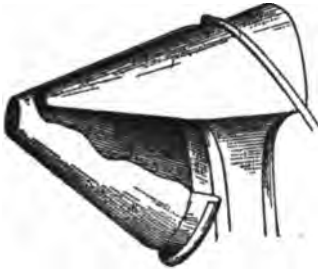
FIG. 149.—PUTTING IN WIRE.
