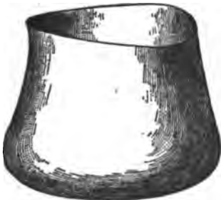
FIG. 169.—SLACK LEFT FOR FORMING LIP.
