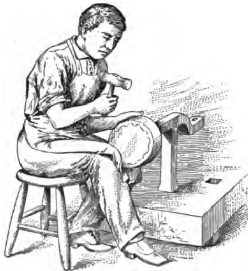
FIG. 107.—PLANISHING TEA-KETTLE SIDE.
