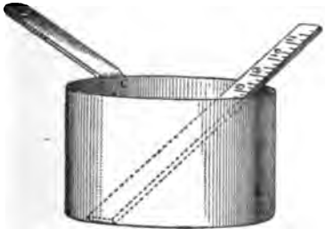
FIG. 15.—MANNER OF MEASURING TO DETERMINE PRICE.
