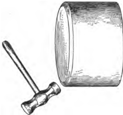
FIG. 175.—FINISHING A SQUARE LAG.
