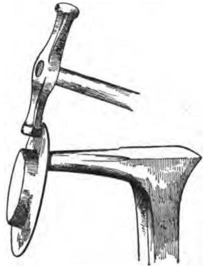
FIG. 142.—PLANISHING COVER ON SIDE STAKE.
