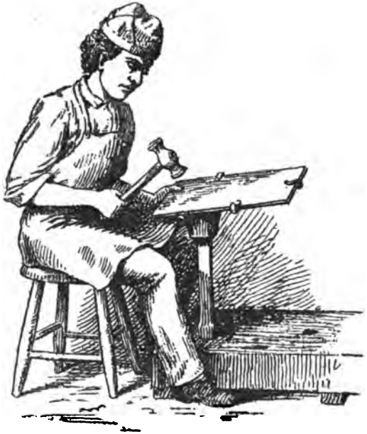
FIG. 19.—PLANISHING AT THE BLOCK.
