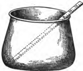
FIG. 164.—BRAZIER'S WAY OF MEASURING SAUCEPANS, ETC.
