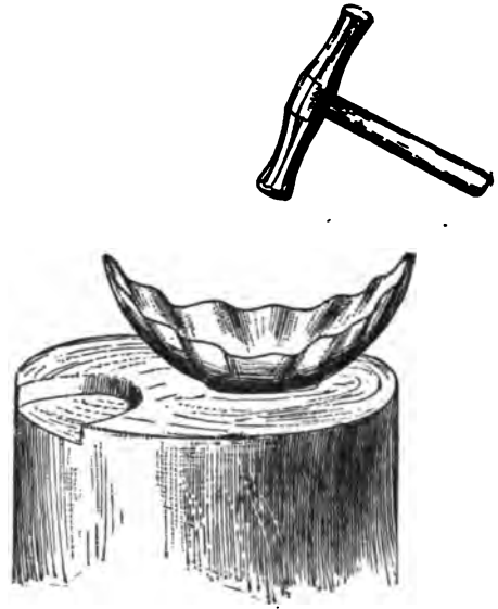
FIG. 253.—SINKING THE CENTER FOR THE BRIDGE.
