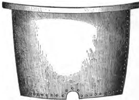
FIG. 454.—SIDES READY FOR RIVETING.
